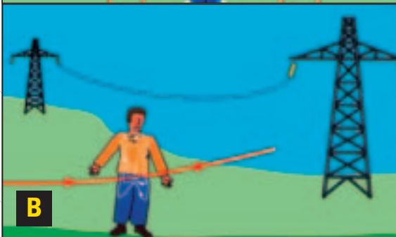
FIGURE 2. A Electric fields do not penetrate the body significantly but they do build up a charge on its surface, while B exposure to magnetic fields causes circulating currents to flow in the body.
